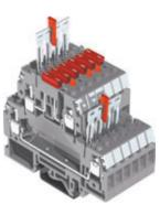
DSFA.4 - detail of the terminal blocks with CNU/8 and SNZ/60 numbering, blade fuse, view of the PTC/4 jumpers on the upper level (upstream the fuse) and on the lower level. The terminal block can be supplied with a nonpolarised LED signal circuit, to detect the fuse blow-out status. Two versions are available depending on the different supply voltages.
